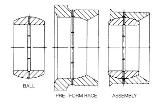
**Figure 8** demonstrates an alternative swaging method used when the bearing geometry precludes or renders impractical the double swaging method shown in figure 7. The pre-form design is used when the bearing outer race is not symmetrical about the spherical centerline due to a flange or a wide overhang on one side or a combination of both. In such case, the problem side of the race is pre-formed by machining and grinding and the opposite side only is swaged.
