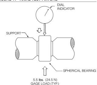
FIGURE 42 - METHOD OF MEASURING RADIAL PLAY
