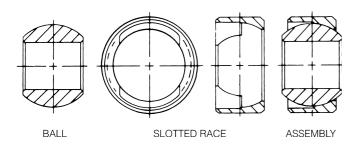
FIGURE 9 - LOADER SLOT BEARING
