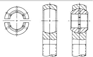
FIGURE 6 - 2- PIECE, SPLIT BALL ROD END
