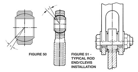
Figure 51 illustrates how misalignment angles for standard ball spherical bearings and rod ends are represented in NMB catalog. The misalignment angle is calculated per Figure 46 formula. Neck ball (high misalignment) bearings and rod ends are represented
