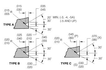
FIGURE 35 - STANDARD V-GROOVE TYPES & SIZES
