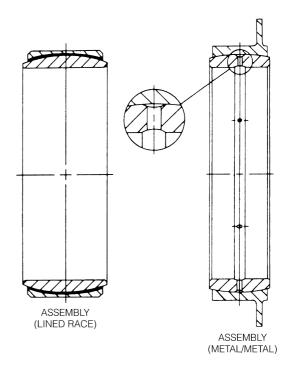
FIGURE 11 - SNAP-ASSEMBLED BEARINGS
