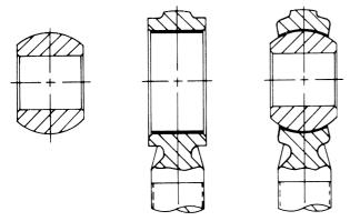
Figure 2 represents Mohawk configuration. The Mohawk 2-piece design is an economical rod end serving a broad spectrum of commercial application. Figure 2 shows the configuration used for Teflon lined Mohawks. This design has good ball to race conformity and can be used in dynamic applications when loads are relatively light.
