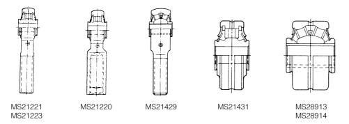
**Figure 15** shows various MS series of roller bearing rod ends and bearings NMB roller bearings are approved for procurement to AS8952 & AS8914 and MS21221, MS21223, MS21220, MS21429, MS21431, MS28913 and MS28914.
