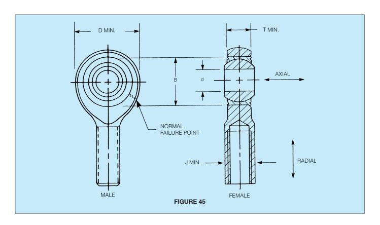
Rod end bearing load ratings can be generated only after carefully determining the load restrictions that each element of the rod end bearing imposes on the entire unit. It order to generate a frame of reference, consider the rod end bearing as a clock face, with the shank pointing down to the 6 o'clock position. The limiting factors in rating a rod end bearing are as follows:
