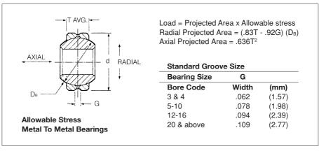
FIGURE 44 - Static load rating formulas for metal to metal spherical bearings.
