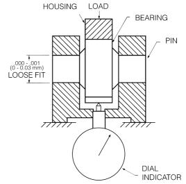
**FIGURE 40 - RADIAL TEST FIXTURE**
