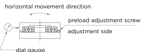
7. Move the slideway to one travel end and slightly lock adjustment screw above the curved roller cage (figure 3-5).
